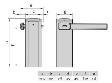
Range of professional electromechanical barriers with inverter and asynchronous three-phase motor for frequent use. Suitable for controlling gates between 2 and 6 metres in width, with fully accessorised bar in a single model. Cap with RGB lights (optional) to serve as traffic light, indicate availability of parking places and for self-diagnosis.
